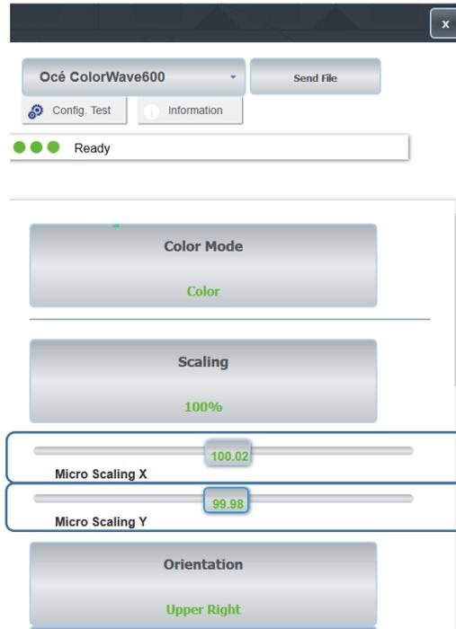
**Fig. 2: Micro Scaling Slider**
